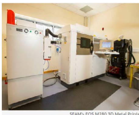
SEAM's EOS M280 3D Metal Printer
