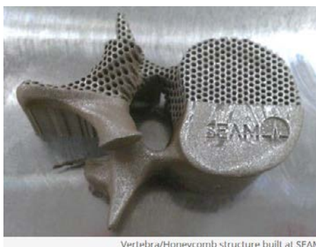
Vertebra/Honeycomb structure built at SEAM
