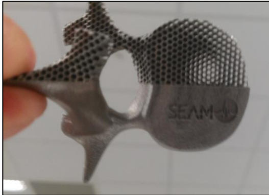
Vertebra/Honeycomb component produced in SEAM via AM
